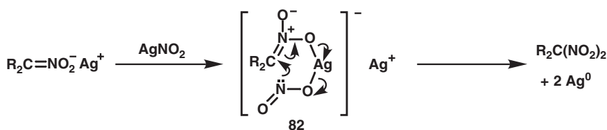
Figure 1.34 Proposed mechanism for oxidative nitration (ref. 105)
